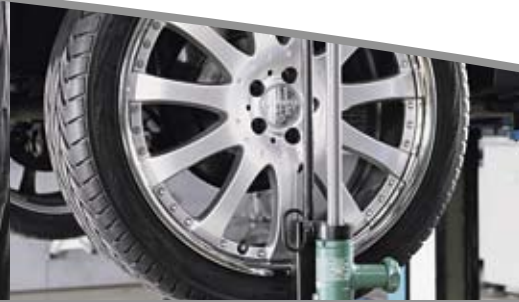
Easy access to wheel bolts. The wheel is positioned away from the main piston.
