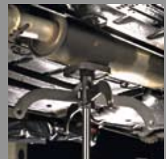
Reversible transmission adaptor improves access when used for jobs other than transmissions.
