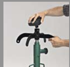
Reversible transmission adaptor with saddle and rubber pad.
